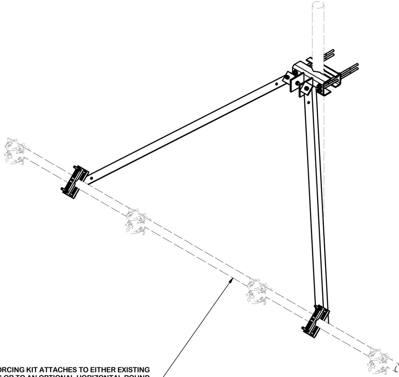
SECTOR FRAME REINFORCING KIT ATTACHES TO EITHER EXISTING SECTOR FRAME CROSS ARMS OR TO AN OPTIONAL HORIZONTAL ROUND MEMBER (SHOWN, SOLD SEPARATELY). IF PURCHASING OPTIONAL HORIZONTAL ROUND MEMBER, CORRESPONDING CROSSOVER PLATE KITS WILL NEED TO BE PURCHASED, ONE PER EXISTING ANTENNA MOUNTING PIPE.
