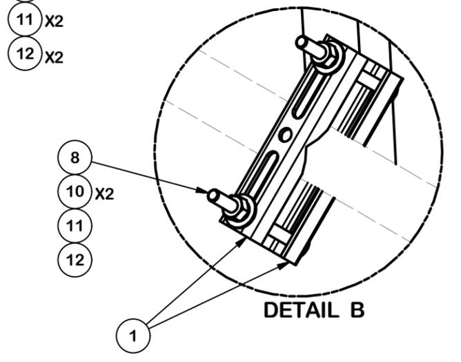
SECTOR FRAME REINFORCING KIT ATTACHES TO EITHER EXISTING SECTOR FRAME CROSS ARMS OR TO AN OPTIONAL HORIZONTAL ROUND MEMBER (SHOWN, SOLD SEPARATELY). IF PURCHASING OPTIONAL HORIZONTAL ROUND MEMBER, CORRESPONDING CROSSOVER PLATE KITS WILL NEED TO BE PURCHASED, ONE PER EXISTING ANTENNA MOUNTING PIPE.
